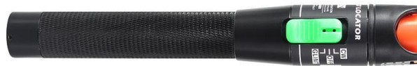
Figure 4.2: Fibre laser pen, or visual fault locator. Injects visible laser beam into fibre, which allows basic alignment and mode matching.
