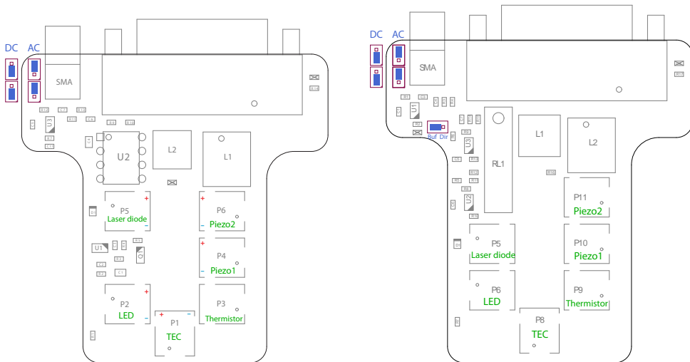
Figure B.3: B1047 (left) and B1240 (right) enhanced laser head boards. Jumpers at top left can be configured for AC or DC coupling. The B1240 has an additional jumper “Buf Dir” for buffered or direct input, shown connected for buffered; change to pins 1 and 2 for direct. Modulation input via SMA connector, sensitivity 2.5 mA/V. Connectors are Hirose DF59.
