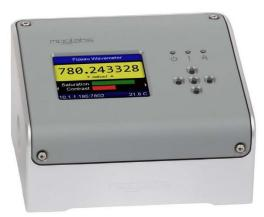
The MOGLabs FZW Fizeau Laser Wavemeter is a precision compact self-contained wavemeter: *no host computer required*.
